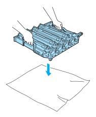
5 Hold the handle of the toner cartridge and pull it out of the drum unit. Repeat this for all of the toner cartridges.
